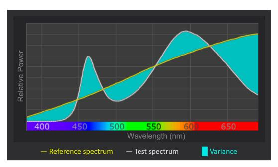
**FIGURE 2.** A graph of the spectral power distributions of both studio tungsten light ("Reference spectrum") and a white LED source ("Test spectrum"), and the variance between them.
